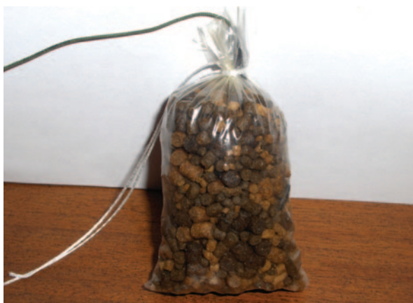
5. Cover the lead with pellets and twist the top of the bag until the bag is fully compressed and tie off using PVA string.
